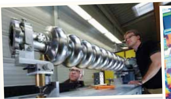
After the sheets have been formed into resonators, they have to pass further quality tests.
