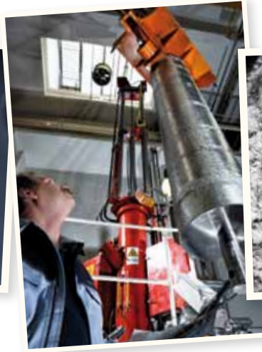
A niobium cylinder weighing tonnes must pass through the smelting facility six times before it is considered pure enough to be processed further.
