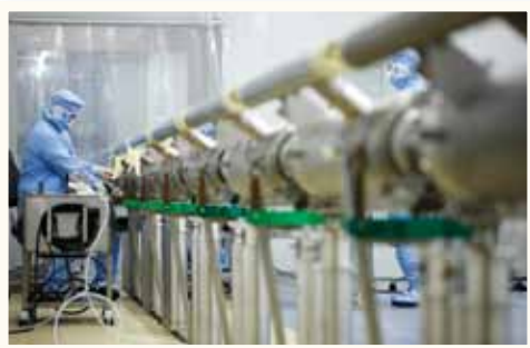
The individual resonators are gradually becoming a string; eight of them are built into one accelerator module.
