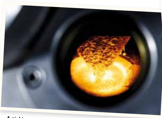
A niobium cylinder weighing tonnes must pass through the smelting facility six times before it is considered pure enough to be processed further.
