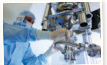
The accelerator elements are assembled in a cleanroom.
