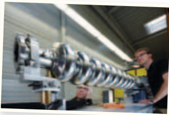
The sheets are formed into accelerator elements.
