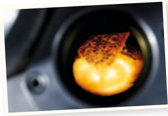
The metal niobium is smelted several times before being processed further.
