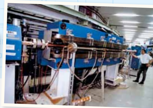
1991: deflecting magnets in the DORIS accelerator
