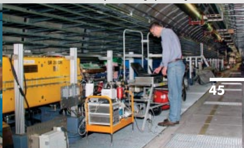
Remodeling finished: 25 meters in front of the collision point, the vacuum chambers for the particle beams already run through joint magnets.
