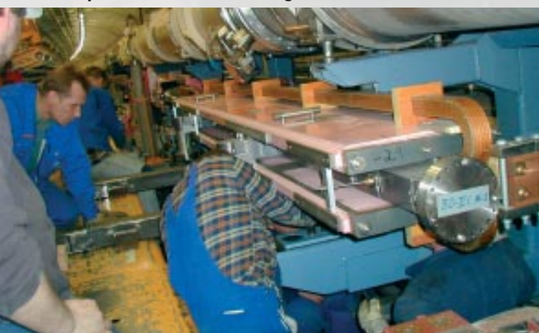
The newly installed spin rotators enable the H1 and ZEUS experiments to utilize the electrons' spin for their own investigations.
